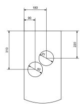
d1 = 120 mm drill hole for cable and lines d2 = 120 mm drill hole for coffee ground ejector
